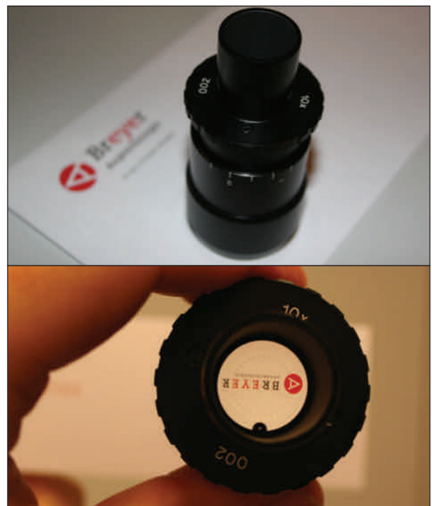
Figure 1. Ocular for the Carl Zeiss Meditec Nd:YAG laser with TABO schema to mark the astigmatic axis on the cornea.
